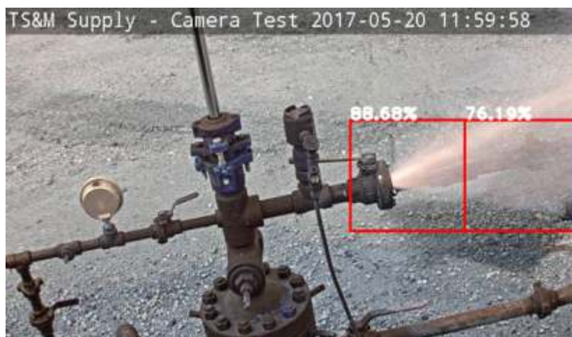
A snapshot of the output of the model localizing the region of leakage.
